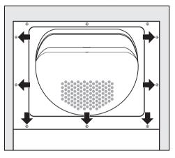
Screw the front panel to the machine door.
